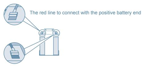
The black line to connect with the negative battery terminal
