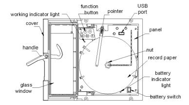
Disc type temperature recorder uses recording paper of the standard 7 inches, record data can be exported by recording paper and U-disk. Please know your temperature recorder well in accordance with the figure above:
